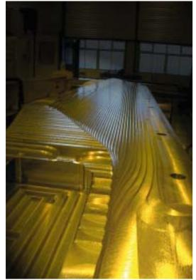
Framework for forming of a reinforcement in honevcomb (Fournier SA)\*
